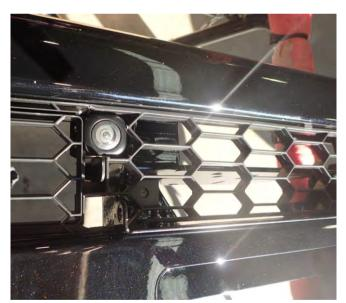
7. Attach camera and bracket assembly to driver's side of winch cradle with M6 hardware as shown.
