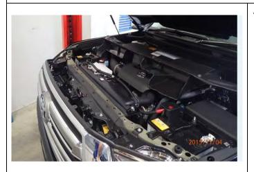
1. Remove plastic engine bay cover above grill area and set aside. Press down on centre of plastic plugs with small screwdriver or similar to release.
