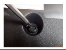
2. Unplug camera then unscrew both phillips head screws and remove from vehicle.
