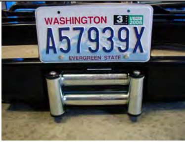
Fitting with winch, number plate above RFL
