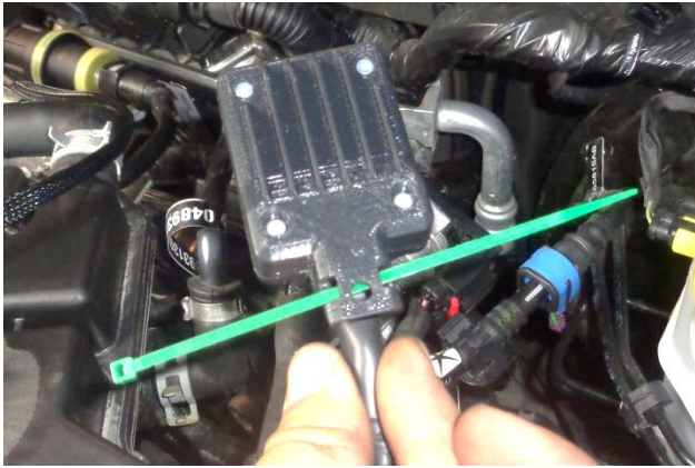
17. Insert a cable tie through the mounting lug on the back of the module housing.
