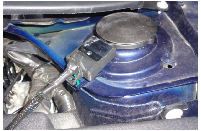
19. Secure the module in a safe location under the hood, such as at the top of the strut tower.
