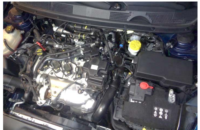
20. Neatly bundle any excess electrical lead, and use the two remaining cable ties to secure the bundles to a safe location (away from moving or hot parts).
