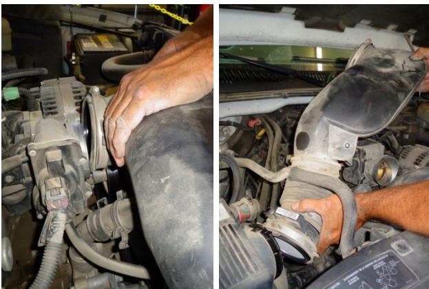
9. Disconnect the intake duct from the throttle body, then remove the duct and MAF sensor from the vehicle.
