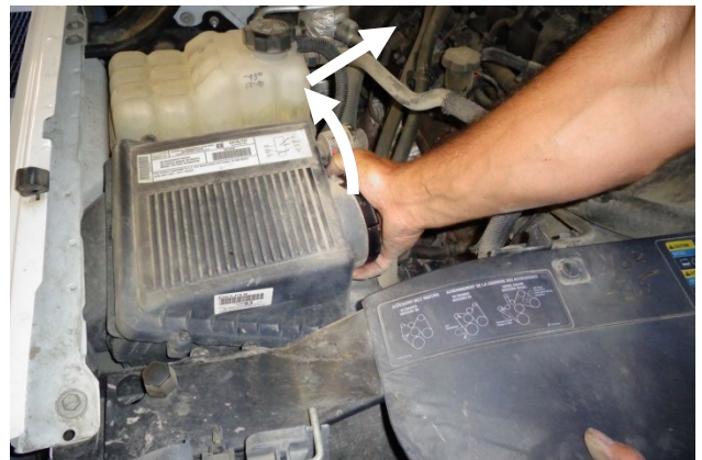
11. Remove the airbox by grasping its inboard side, lifting straight up (to release the mount pins from their rubber grommets), and sliding the airbox inboard to release it from its shelf.
