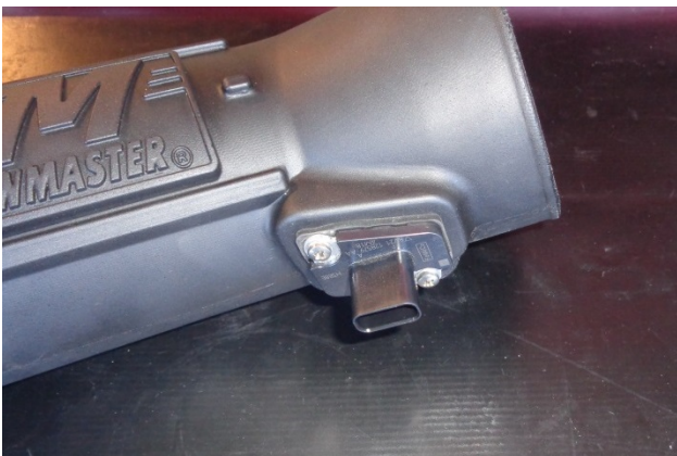
20. Install the MAF sensor gasket (21) onto the sensor, ensuring correct orientation. Then install the sensor in the intake tube, using M4 screws (23).
