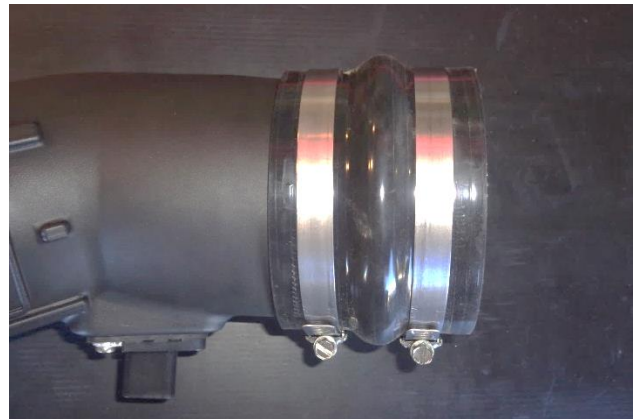
22. Install the two larger hose clamps (19) on the larger coupler (20), and install the coupler on the filter end of the intake tube. Do not tighten clamps at this time.
