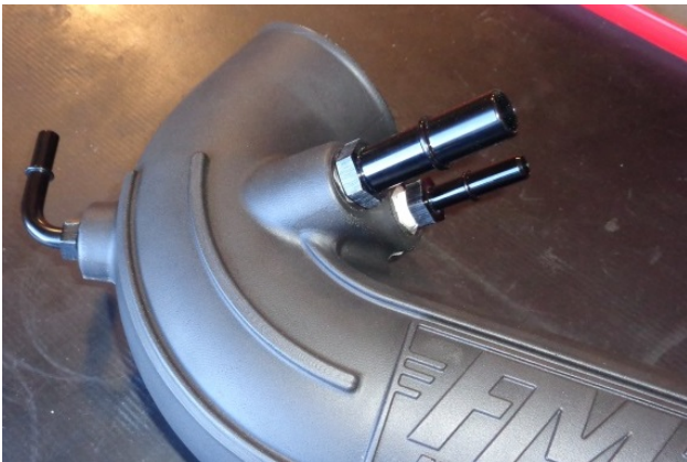
19. Apply 2 wraps of nylon thread tape to the 5/8" QD fitting (25) and the 3/8" QD fitting (22), and install them in the intake tube as shown. NOTE: For best hose alignment, we have located the 5/8" fitting above the 3/8" fitting (which is opposite the stock setup).
