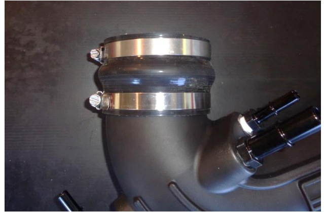
21. Install the two smaller hose clamps (28) on the smaller coupler (27), and install the coupler on the throttle end of the intake tube. Do not tighten clamps at this time.
