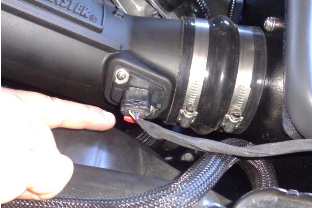
24. Install the MAF sensor plug on the sensor, and push the locking tab toward the sensor. Then check the plug for security.
