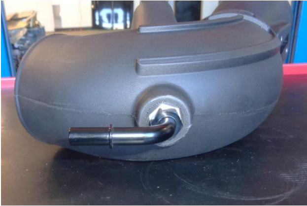
18. Apply 2 wraps of nylon thread tape to the 3/8" quick disconnect (QD) elbow (26), and install it in the intake tube (24). Align the elbow with the tube's mold line as shown.
