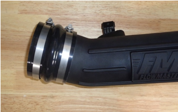
20. The kit includes three large screw clamps (10) and one small clamp (17). Install two large screw clamps on the flex coupler (9), and install the coupler on the filter end of the intake tube. Snug (but do not yet tighten) just the clamp on the tube, and leave the other clamp loose.
