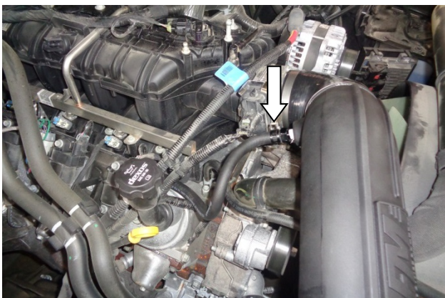
27. Cut the hose to length, and secure the other end to the barbed fitting with the other pinch clamp (15).
