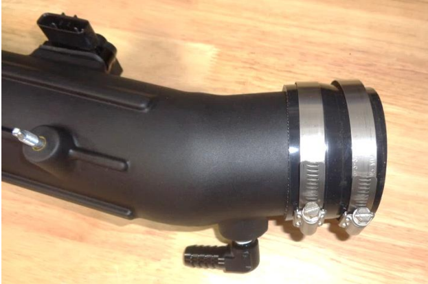
25. Install the 2 small hose clamps (34) on the straight coupler (33), and install the coupler on the throttle body end of the intake tube. Do not tighten clamps at this time.
