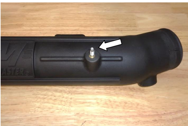
21. Install the engine appearance cover mount stud ( removed at Step 12 ) in air intake tube (25).
