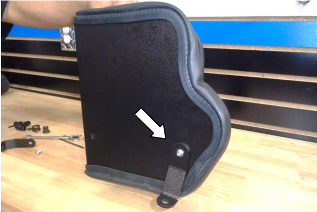
19. Attach bracket (5) to the heat shield using ¼-20 screw (7) (on the bracket side), and flat washer (6), lock washer (8) and nut (9) (on the heat shield side). Do not fully tighten the fasteners at this time.
