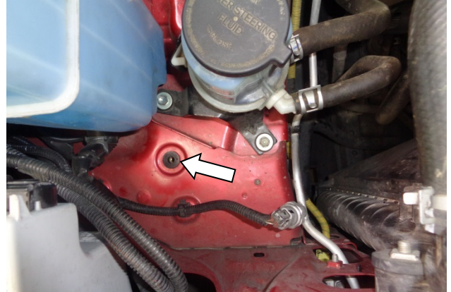
28. Insert rubber well nut (16) in the hole at the front corner of the washer fluid reservoir. (Wetting the well nut with soapy water may ease insertion.)
