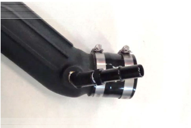
20. Install 2 smaller hose clamps (18) on straight coupler (19), then install coupler on throttle-body end of intake tube.
