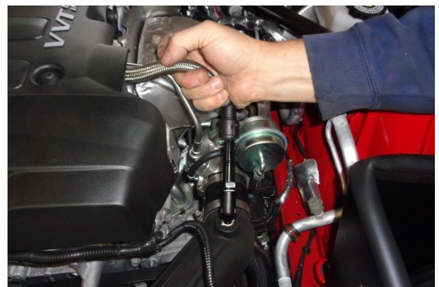
23. Connect the PCV line to the quick disconnect fitting and check for security.
