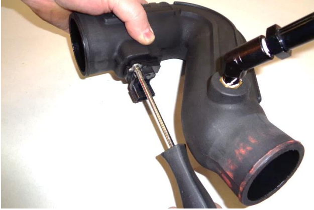
18. Place the MAF sensor gasket (21) over the sensor, ensuring correct orientation. Then install the sensor in the intake tube, using M4 screws (20).
