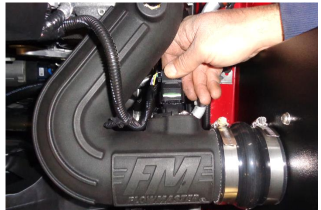
22. Reinstall the connector on the MAF sensor, close the locking tab, and verify that the connector is secure.
