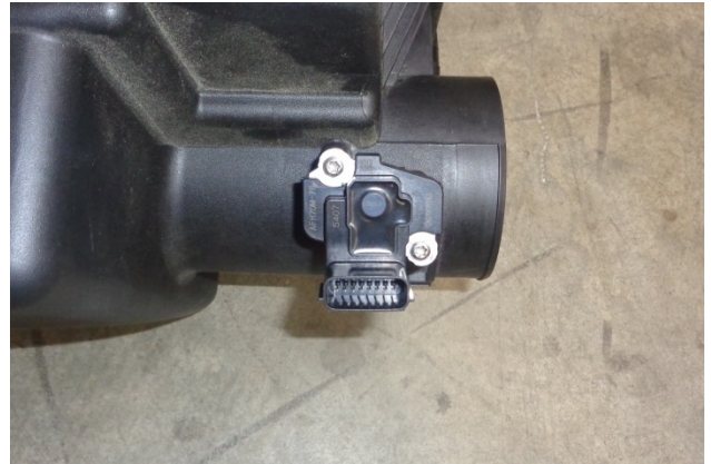
12. Remove the MAF sensor from the airbox, then remove the factory gasket from the sensor. CAUTION: The sensor is delicate! Handle it with care, and store it in a safe location until reinstallation.
