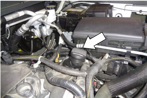
8. Reinstall the oil filler cap.
