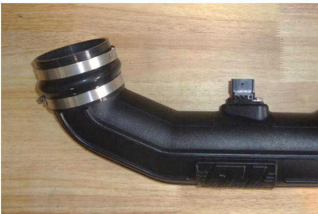
21. Install the two larger screw clamps (16) on the 3-1/2" coupler (17), and install the coupler on the filter-end of the intake tube. Do not tighten the clamps at this time.
