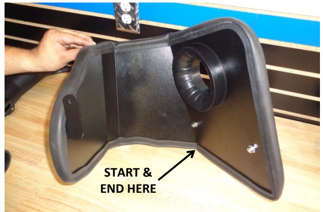
17. Attach the gasket (9) to the heat shield. Starting at the corner shown, firmly press the gasket onto the edge, gradually working around the heat shield. When you return to the starting point, trim the gasket to fit using metal-cutting shears.
