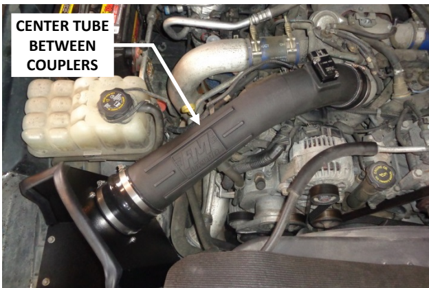
20. Center the intake tube between the couplers (so that there is roughly an equal amount of the tube ends inside each coupler), and tighten the two intake tube clamps.
