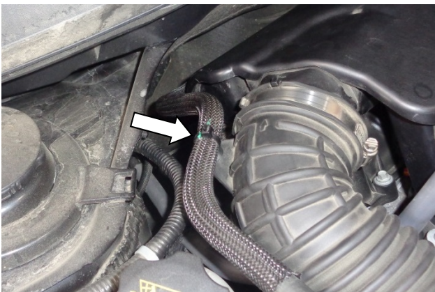
9. Release the hose and clamp from the intake duct.
