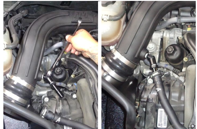
28. Align the elbow and quick connect fitting with the breather hose. Connect the breather hose to the fitting and verify the connection is secure.
