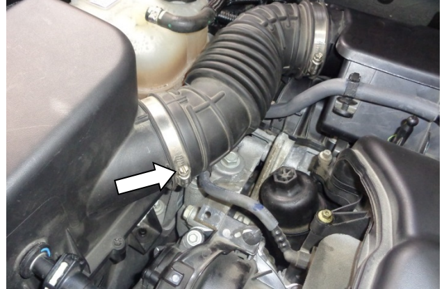
10. Loosen the screw clamp securing the intake duct to the airbox.
