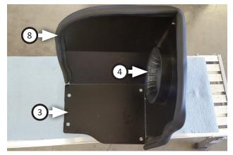
Install air filter adapter (4) into airbox (3) using (x3 ea.) screws (13), split lock washers (14) and flat washers (15). Apply trim seal (8) to airbox then trim excess so it fits precisely as shown.
