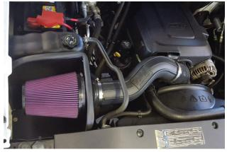
Install cone air filter (1) into airbox, plug MAF back in and if applicable, plug MAP back in. Use zip tie (20) to secure wiring harness, then replace engine cover.
