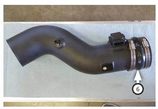
15. Place (x2) hose clamps (7) onto both sides of hump coupler (6), then fit it onto MAF side of intake tube as shown.
