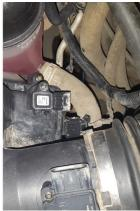
3. Unplug MAF sensor from factory airbox. If applicable, also unplug MAP sensor.
