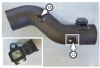
14. Install hose barb (18) into intake tube. Then either install sensor block off plate (11) using screw (13) or, if applicable, install MAP sensor (removed step 9) near MAF sensor.
