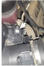
9. Remove and retain MAF sensor from factory air box. If applicable, remove MAP sensor from air box beside MAF sensor where shown.
