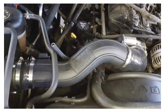
19. Place intake tube assembly into engine compartment and center tube between coupler and throttle body.
