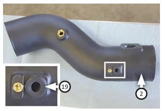
11. Install grommet (19) into intake tube (2).
