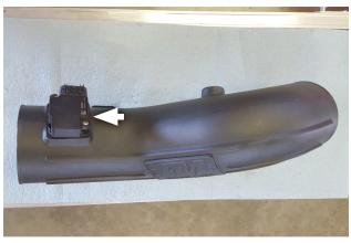
13. Install MAF assembly onto intake tube.
