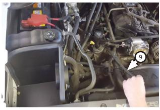
18. Set (x2) pinch clamps (17) onto fuel hose (9) then install one end onto crank case vent and move pinch clamp over connection.
