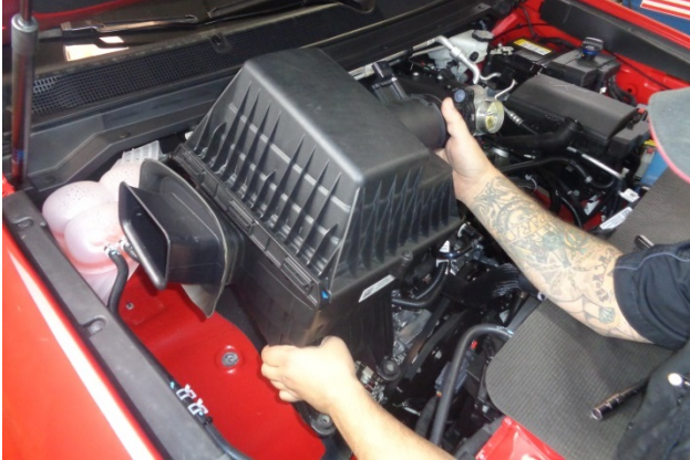
13. Firmly lift the airbox straight up and remove it from the vehicle.
