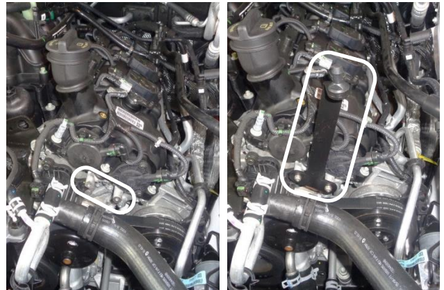
23. Locate the 2 screw holes on the engine as shown, and attach the bracket using M6 screws (8), lock washers (7) and flat washers (6).
