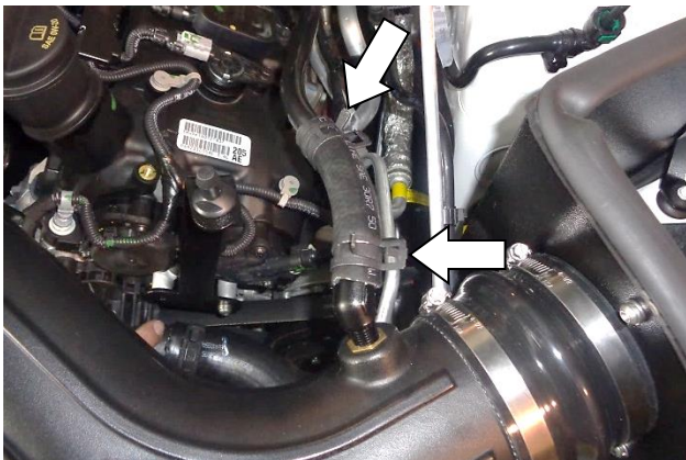
32. Push one end of the 5/8" I.D. hose (23) onto the PCV tube. Cut the hose to fit the barbed fitting in the intake tube, and secure at both ends using pinch clamps (22). NOTE: Point the ears on the clamps toward the heat shield, so that they do not hit the engine cover when it is installed at Step 35 .
