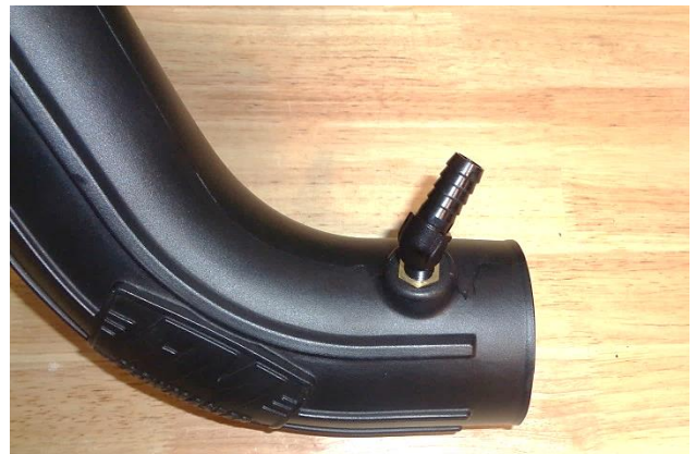
24. Apply 2 wraps of nylon thread tape to the threads of the barbed elbow (21), and install it in the intake tube (20).
