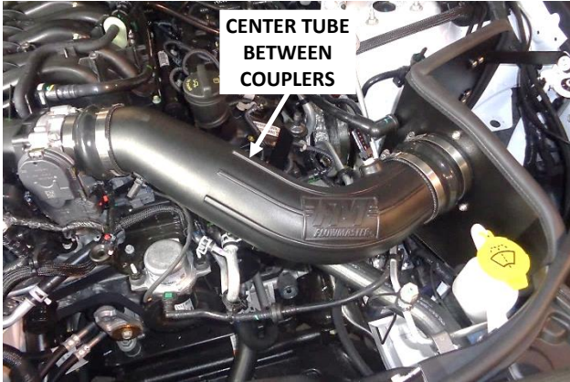
31. Center the intake tube between the couplers (so that there is roughly an equal amount of the tube inside each coupler), and tighten the two intake tube clamps.
