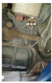
5. Remove and retain fasteners from inlet pipes then disconnect and remove muffler sections from vehicle.
