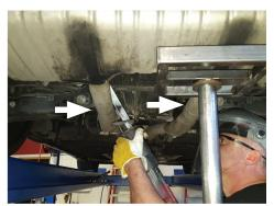
4. Dismount both front wire hangers, remove nuts (x4) and muffler/pipe hangers (x2) from muffler rear then disassemble and set aside muffler from vehicle. Retain nuts and muffler/pipe hangers for later use.
