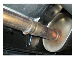
3) Support the muffler with a stand and loosen the clamp on the muffler inlet pipe, then remove the two hangers at the rear of the muffler from the rubber mounts on the vehicle. Slide the muffler to the rear and disconnect from the inlet pipe. Lower and set the muffler aside.
