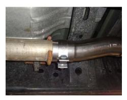
1) Place the provided 3" clamp onto the inlet of muffler **#72198-505**, then slide onto the factory front pipe and connect the two hangers at the back of the muffler to the rubber mounts on the vehicle. Be sure to line up the notch on the muffler inlet with the tab on the pipe.
