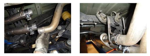
2) Place the provided 2<sup>1</sup>/<sub>4</sub>" clamps onto the muffler outlets and re-install the tailpipes into the muffler outlets. Be sure to line up the tabs on the tailpipes with the notches on the muffler outlets. Tighten the clamp securely.
