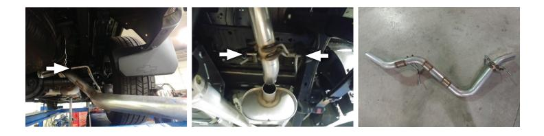
5. Dismount inlet exhaust pipe from mount. Loosen clamp from catalytic converter connection then remove remaining exhaust assembly from vehicle. Remove and retain clamp for later use.
