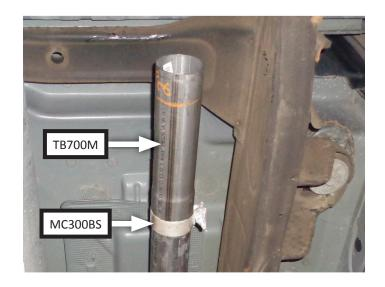
10. Place **3" clamp (MC300BS)** onto **muffler (72149-Z)** inlet then connect muffler to inlet pipe or extension. Tighten clamp just enough to allow for adjustment.
