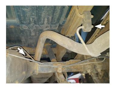
4. Support muffler and remove nuts (x2) from inlet pipe flange. Disassemble wire hangers from isolators and remove exhaust system. Retain nuts for later use.
