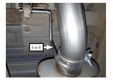
Fasten right frame hanger (8) to vehicle using bolt (11), backing plates (x2) (10), flat washer (13), lock washer (14) and nut (12) as shown. Then hang rubber hanger (9) on frame hanger end.
