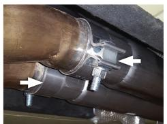
4. Carefully lower stands at vehicle rear and with help from an assistant, slide system back off the head pipes and lower system from vehicle.
