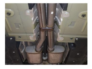
12. Place clamps (x2) (MC300BS) onto right and left tailpipe (26626M, 26628M) inlets then connect tailpipes to muffler outlets. Connect wire hangers to rubber isolators and adjust tailpipes so that tips are level and centered in bumper cut-out. Tighten clamps just enough to allow for adjustment.
