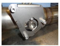
Insert screws (x3) (HW240) through actuator and flat washers (x3) (HW315). Place actuator onto tailpipe valve mount then tighten screws to fasten assembly. CAUTION: Make sure you place flat washer between actuator and standoff as shown, **NOT** beside screw head.
