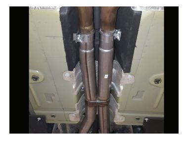
11. Place clamps (x2) (MC300BS) onto FFX muffler (x2) (71229-Z) inlets. Slide mufflers onto scavenger pipe about 1¾" then level them. Tighten clamps just enough to allow for adjustment.
