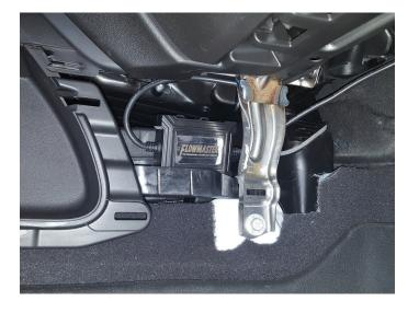
18. Remove wire, tape and lubricant from controller kit. Thread wire end down and connect it to wire assembly. Secure any slack away from moving and heated engine components.
