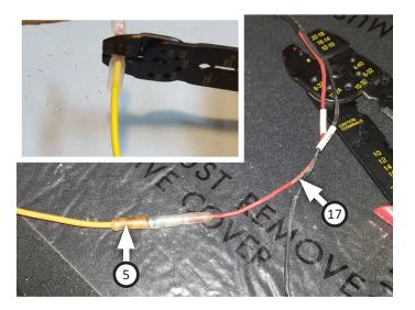
13. Place **female quick disconnect (16)** to remaining end of controller kit. Crimp connector to secure wires together.
