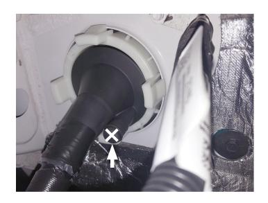
15. Thread hanger wire into cab through firewall, then bend its end and connect it to controller kit. Tape over connection to secure it.
