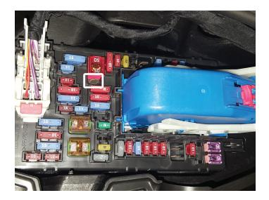
20. Connect female quick disconnect end of controller kit to fuse box.
