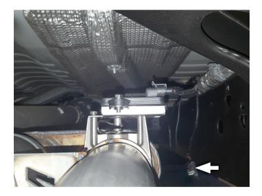
**NOTE:** You may secure wire assembly several different ways; **zip tie (13)** it to factory wire bundle, tuck it behind heat shield, secure it to frame, etc. Just be sure that connections are stable and wire is protected from heat.
