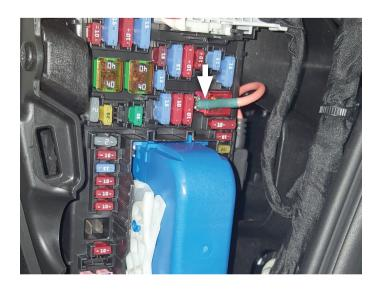
21. Connect ground wire of controller kit to metal frame under dashboard using **bolt (10)**, **flat washers (x2) (12)** and **nut (11)** as shown. Tuck any slack cord up and out of the way of vehicle operation.
