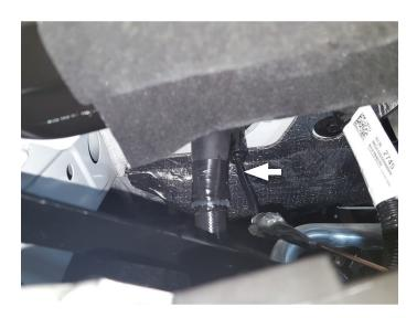
17. Fasten controller kit to a point up and away from interfering with passengers feet.
