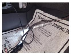
16. Cover connection with lubricant then pull hanger wire back through firewall into engine bay.
