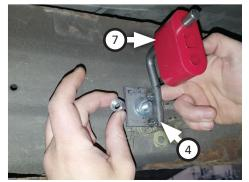
8. Place factory ball clamp (removed step 4) onto **inlet pipe (1)** then connect it to cat. converter. Insert wire hanger in isolator and tighten clamp enough to allow for adjustment.
