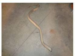
4. Disassemble wire hanger from isolator, loosen ball clamp and remove muffler section. Release tab to remove ball clamp from pipe and retain it for later use.
