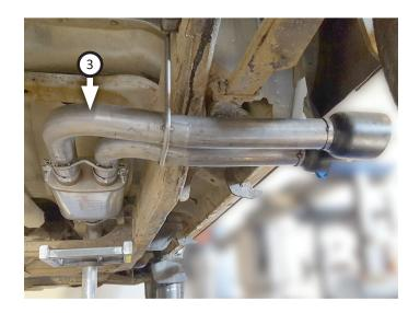
11. Adjust exit pipe until tips are desired distance from body, then lay bracket flat against vehicle rail and mark holes (x2). Rotate bracket away, drill marks with a ¼" drill bit then secure bracket to rail using (x2) **bolts (9)**.
