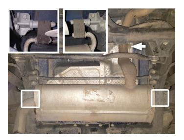
4. Loosen ball clamp from resonator inlet, disassemble hanger wires from isolators and remove resonator section from vehicle. Release tab to remove clamp from pipe and retain it for later use.
