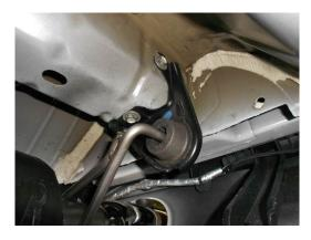
3) Using a 13mm wrench, loosen the two hangers just behind the rear differential from the cross member and the two hanger mounts at the rear of the vehicle from the frame. Slide the muffler assemblies toward the rear of the vehicle to disengage them from the factory system. Leave them hanging in place for re-assembly onto the Flowmaster X-pipe assembly.
