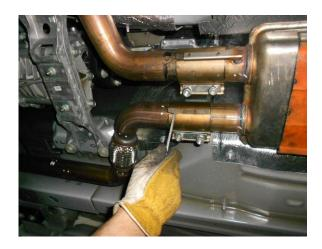
3) Support the center resonator with a stand and loosen the four nuts at the two band clamp connections at the resonator inlet. Using a screwdriver, pry up the clips on the clamp body to release the clip from the tab on the inlet pipes. Slide the clamp assemblies slightly back to clear the tabs. You can now lower the rear of the resonator and slide the assembly to the rear of the vehicle to remove. Lower the resonator from the vehicle and set aside.
