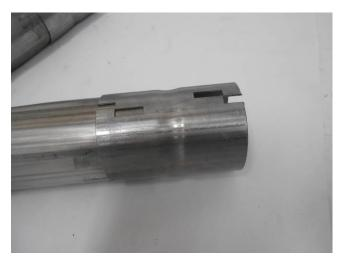
1) Slide a supplied **TB810S** adapter pipe onto the end of each outlet of the 86348 X-pipe assembly. Place a supplied clamp onto the connections and tighten enough to hold.
