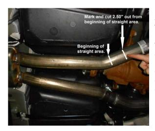
2) Begin by measuring back 2 ½" from the beginning of the straight area shown in the photo at left and make a mark on both pipes. Support the exhaust system both in front and behind the area to be cut. Check that the marks are correct, then using a sawsall, cut both pipes at the marks. Note: Due to the closeness of the pipes to the gas tank, use caution when cutting! Carefully deburr the end of the muffler inlet pipes where cut with a file or die grinder.
