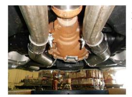
2) Place a stand under the center resonator just forward of the axle-back muffler assemblies. Loosen the clamps at the inlets of the Flowmaster axle-back mufflers.
