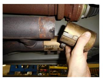
3) Use a **15mm** socket to loosen the nuts on the two clamped connections in the center of the vehicle behind the factory H-pipe on GT models, and X-pipe on GT500 models. Remove the intermediate pipes and set aside. To make the installation of the right side over-axle pipe easier, remove the factory clamp on the right side of the exhaust by lifting the clip on the clamp with a screwdriver. Place the clamp onto the front of the right over-axle pipe in preparation for the next step.
