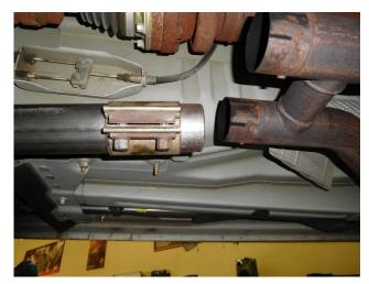
1) Place the new right side intermediate pipe #86397S with the factory clamp installed into position over the rear axle and onto the back of the factory H-pipe/X-pipe. Repeat this step on the left side of the vehicle with intermediate pipe #86398S.
