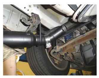
2) Place a 2.50" clamp onto the inlet pipes of both muffler assemblies. Slide the mufflers (with hanger mounts in place) onto the over-axle pipes, and support with stands. Secure the hanger mounts back into position on the frame using the factory bolts. A **13mm** ratcheting box-end wrench works best to reach the bolts above the muffler. Tighten the clamps on the muffler inlets enough to hold but still allow for adjustment.
