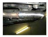
8) Place tailpipe assembly **#16755S** up over the rear axle and into the muffler outlet. Connect the hanger at the rear of the pipe to the rubber mount on the vehicle. Adjust the tip to the desired rotation and tighten the clamp enough to hold but still allow for adjustment. **Note:** Depending on the model year and or spare tire size, the spare tire may need to be dropped down to allow installation of the new Flowmaster tailpipe.
