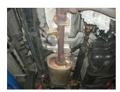
4) Support the muffler with a stand and separate the four hangers on the muffler and front pipe assembly from the rubber mounts on the vehicle. Lower the stand and remove the assembly from the vehicle.
