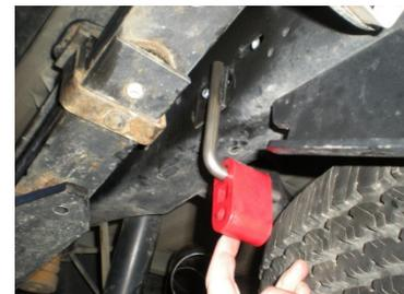
10) Place a provided 4" clamp onto the expanded end of pipe **#46174S**, connect the hanger on the pipe to the rubber mount installed in the step above. Then connect the front of the pipe to the rear of pipe **#46172S**. Confirm that the two pipes are fully slid together and tighten the clamp enough to hold, but still allow for adjustment.
