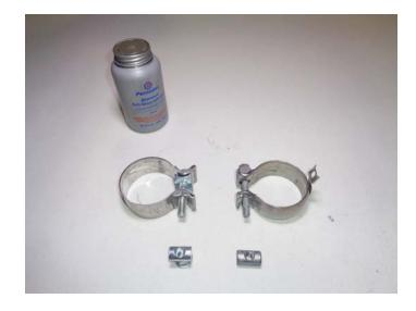
Replace mounts using (x2) front frame hangers (6) and (x4) bolts (removed step 3). Then install (x2) rubber hangers (10) onto front frame hangers.
