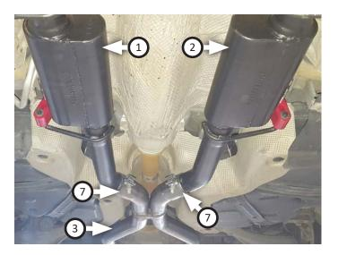
Use (x2 ea.) bolts (8), steel spacers (9), flat washers (12), springs and nuts (removed step 3) to fasten right and left resonators to factory flanges then tighten clamps enough to allow for later adjustment. **NOTE:** Tighten fasteners until nuts bottom out on steel spacer sleeves.
