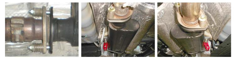
Place clamp (7) onto left muffler assembly (4), connect it to left side scavenger outlet, insert wire hangers into isolators then tighten clamp enough to hold parts. Repeat step with right muffler assembly (5).
