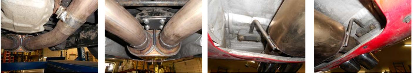
9) Adjust the position of all pipes and muffler to provide a satisfactory fit. A minimum 3/4" clearance around all parts of the system must be maintained; while also keeping suspension travel and vibration in mind. Tighten all clamped connections down securely. For a more secure installation, we recommend welding all slip-fit connections.
