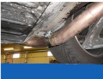
6) On the right side of the vehicle, place a provided 3" clamp onto the expanded end of mid pipe assembly **26443S**. Route the pipe up over the frame and connect to the back of front pipe **26441S**, rotate the pipe to achieve equal clearance around the pipe and tighten the clamp enough to hold, but still allow for adjustment. Re-install the O2 sensor removed in step 4 above into the fitting on the new Flowmaster pipe. Repeat this step on the left side with pipe **#26444S**.
