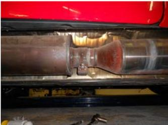
2) Using a penetrating lubricant, spray the rubber hangers that support the exhaust system from the catalytic converters back. Also, spray the nuts on the clamped connections behind the catalytic converters as well as the two just forward of the rear muffler assembly. This will greatly ease the removal of the system.
