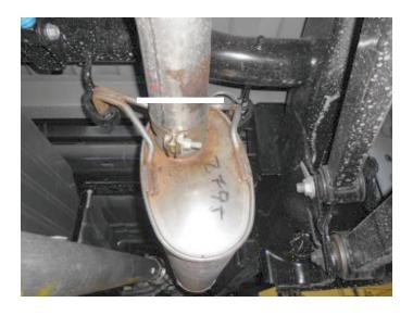
4. Support muffler and remove all hangers from isolators on muffler assembly; then remove clamp on slip connection just behind catalytic converter. Heat or cut to separate connection and remove muffler assembly.
