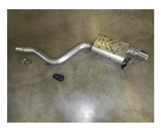
1) Place the new Flowmaster muffler units next to the factory units and swap the front and rear hanger mounts from the stock mufflers to the Flowmaster assemblies. Also, place a provided 2.50" clamp onto the inlet of each assembly. Tighten the clamp just enough to hold in place.
