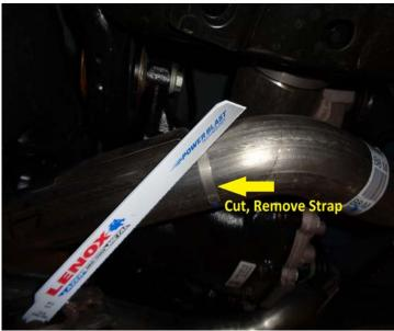
3) Begin by removing the two pipe heatshields indicated in the first picture above. Cut thru the strap at the rear of the shield, then lift and lower the shield a few times to break the weld at the front of the shield. Remove.
