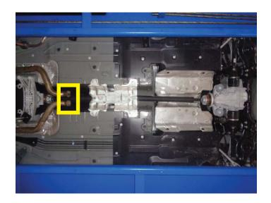
8. Remove nuts (x3) then detach actuator and spring from mount on driver side tailpipe. Retain actuator and spring for re-use. Repeat step for passenger side tailpipe.
