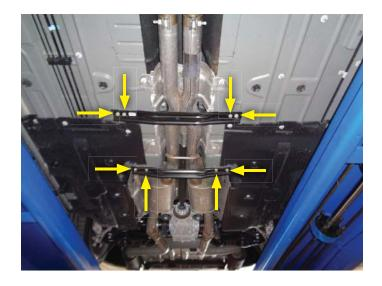
7. Loosen clamps (x2) connecting factory exhaust system to front pipes. Carefully slide system off of front pipes to remove completely from vehicle.
