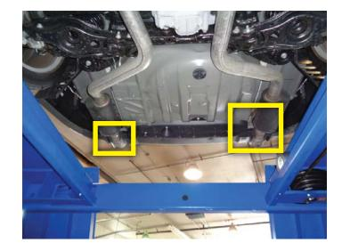
4. Unplug wire from driver side exhaust valve actuator. Repeat step for passenger side exhaust valve actuator.
