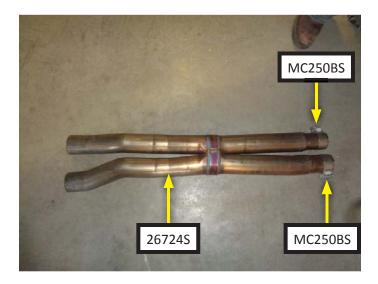
14. Slide scavenger pipe into front pipes then tighten both clamps just enough to allow for adjustment. Tighten nuts (x8) to install braces which support scavenger pipes. (removed step 6)
