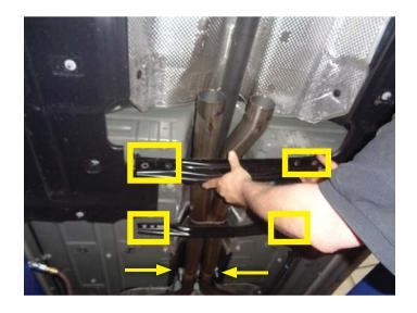
15. Install clamps (MC300BS) (x4) onto both mufflers (15430-253).
