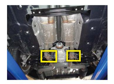
5. Unclip grounding strap and slide wire hanger out of rubber isolator on driver side tailpipe. Next, unbolt mount, flip it around and reinstall. Repeat step for passenger side tailpipe.
