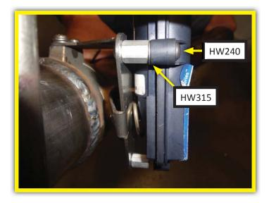
12. Place factory mount from driver side tailpipe onto left tailpipe. Repeat step for right tailpipe. (removed step 1)
