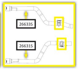
11. Place driver side actuator onto left tailpipe valve bracket. Place **flat washers (HW315)** (x3) between actuator and standoff then loosely fasten **3/4**" **screws (HW240)** (x3). Once actuator is located, finish tightening all screws. Repeat step for right tailpipe. (removed step 8)
