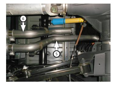
12. Place clamp (15) on left rear tailpipe (7) then connect it to left front tailpipe at slip-fit connection over rear axle. Place rear hanger into rubber hanger then tighten clamp just enough to allow for adjustment.
