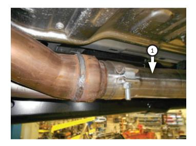
8. Place clamp (14) onto extension pipe (2 or 3) then connect it to inlet pipe. Connect wire hangers to isolators then tighten clamp just enough to allow for adjustment.
