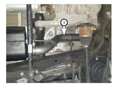
9. Place **clamp (5)** onto **exit pipe (4)** then connect it to overaxle pipe. Insert wire hanger into isolator then tighten clamp just enough to hold parts.
