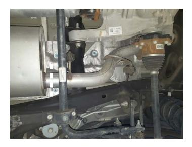
4. Support muffler and disassemble wire hangers from isolators. Loosen ball clamp, disconnect inlet pipe at cat. converter and remove exhaust system. Release tab to remove clamp from pipe and retain it for later use.
