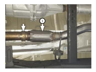
7. Place clamp (5) onto muffler (2) then connect it to inlet pipe. Tighten clamp just enough to allow for adjustment then place clamp (5) onto muffler outlet.
