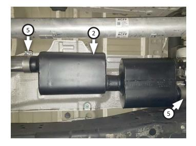
8. Route **overaxle pipe (3)** over axle then connect it to muffler. Insert wire hangers into isolators then tighten clamp enough to allow for adjustment.
