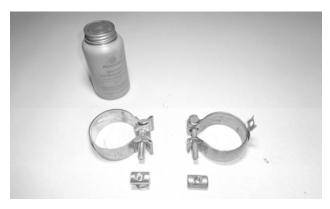
**7. Before installing any clamps,** remove their nuts, apply antiseize compound to the bolt threads, and re-install the nuts.
