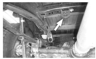
**5.** Remove the isolators from the muffler, then reinstall the rear isolator on the frame. (One front isolator will be installed later.)
