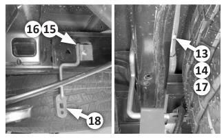
6. On the driver's side frame (between the leaf spring and spare tire), install frame hanger (15) using the 3-1/2" bolt (16) (on outside of frame), and backing plate (17), lock washer (14), and nut (13) (on inside of frame). Lightly snug the fasteners (to allow final adjustment later). Lastly, slide rubber hanger (18) onto the rod.
