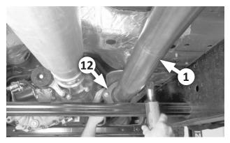
9. Slip flange (12) over the head pipe (1), then attach the head pipe to the catalytic converter flange using the stock fasteners. Lightly snug the fasteners (to allow final adjustment later).
