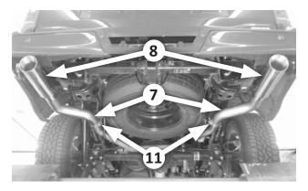
17. Slip a 2-1/2" clamp (11) over each rear exit pipe (7), and install each one on its tail pipe. Align each exit pipe as desired, verify 3" of insertion, and snug each clamp slightly. Install a tip (8) on each rear exit pipe. Align each tip as desired, and tighten its clamp.
