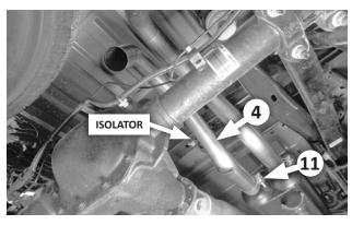
15. Slip a 2-1/2" clamp (11) over the muffler's left outlet. Move the left over-axle pipe (4) into place, slide its hanger rod into the isolator, and slip the end of the pipe into the muffler's outlet. Verify 2" of insertion, then snug the clamp slightly.
