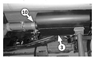
**13.** Slip a 3" clamp (10) onto the head (or extension) pipe. Slip muffler (3) onto the pipe, support it with a stand, verify 2" of insertion, and snug the clamp slightly.
