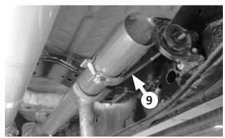
**12. Slide clamp hanger (9)** over the head (or extension) pipe. Slip a front isolator over the hanger rod, and use the stock screws to attach it to whichever frame location gives the best fit for your truck. Snug the screws and clamp lightly (to allow final adjustment later).
