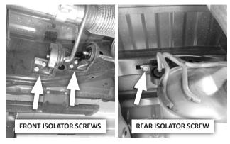
**4.** Remove the screws from the muffler's front and rear isolators. Then remove the assembled inlet pipe, muffler, and isolators from the vehicle.
