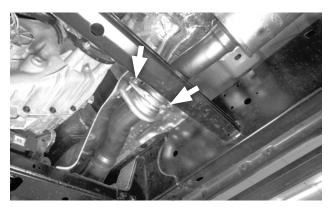
3. Remove and retain the 2 fasteners from the inlet pipe flange.
