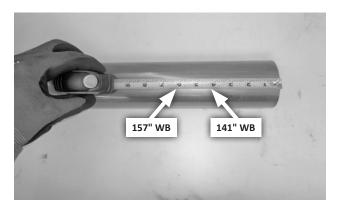
**8. FOR 141" AND 157" WHEELBASE TRUCKS:** Cut the head pipe back as specified in **Step 7.**
