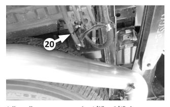
18. Adjust all components to give 1/2" to 3/4" clearance (about a finger's width) around them, and allowing for suspension travel and vibration. (If necessary, relocate the front isolator and clamp hanger, installed at Step 12.) When you are satisfied with the system's clearance and fit, tighten all clamps and hardware. Use cable tie (20) to keep electrical and fluid lines away from exhaust components.
