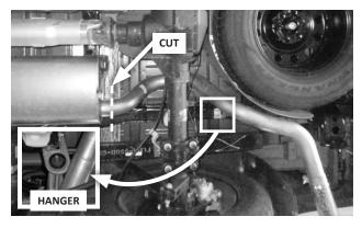
2. Cut the tailpipe off just behind the muffler. Disengage the tailpipe's hanger rod from its rubber isolator, and remove the tailpipe from the vehicle.
