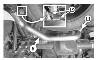
16. Slip a 2-1/2" clamp (11) over the front of the left tailpipe (6), and move the pipe into place. Slip it onto the left over-axle pipe, slide its hanger rod into the rubber hanger installed at Step 6, and install the two hanger keepers (19). Verify 3" of insertion, and snug the clamp slightly.
