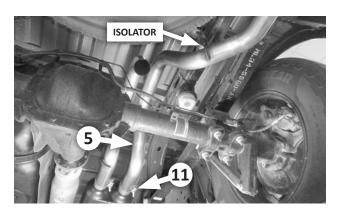
**14.** Slip a 2-1/2" clamp (11) over the muffler's right outlet. Move the right over-axle pipe (5) into place, and slide its hanger rod into the isolator. Then slip the end of the pipe into the muffler's outlet, verify 2" of insertion, and snug the clamp slightly.
