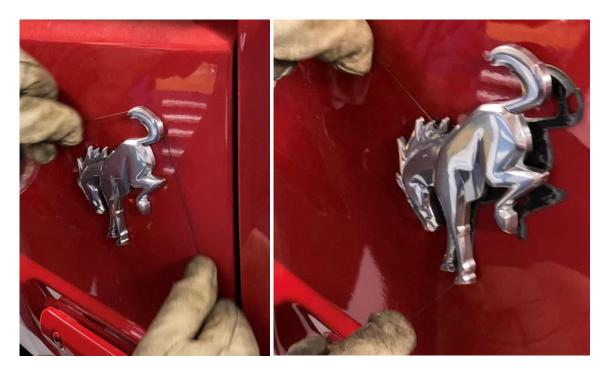
4. Remove the remaining foam and clean surface with alcohol wipes.
