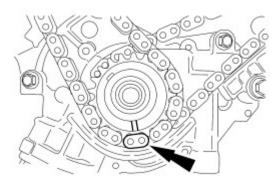
**STEP 15:** Install the RH timing chain onto the crankshaft sprocket, aligning the copper (marked) link with the timing marks on the sprocket.
