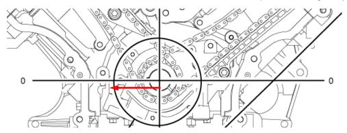
**STEP 2:** With the crankshaft remaining in the 9 o'clock position loosen both camshaft sprocket bolts leaving them loose in the camshafts. While leaving the camshaft bolts loose in the camshafts remove all timing components followed by the camshaft bolts, washers, sprockets, and spacers.
