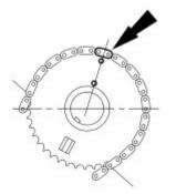
STEP 11: Position the LH timing chain tensioner arm on the dowel pin and install the LH timing chain tensioner. Hand start tensioner bolts and torque to 25 Nm.NOTE: The LH timing chain tensioner arm has a bump near the dowel hole for identification.
