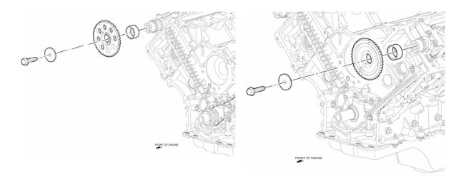
**STEP 6:** Rotate the LH camshaft sprocket until the timing mark is approximately at the 12-1 o'clock position. Rotate the RH camshaft timing sprocket until the timing mark is approximately in the 11 o'clock position.
