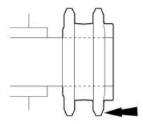
**STEP 9:** Position the LH (inner) timing chain on the crankshaft sprocket, aligning the copper (marked) link with the timing mark on the sprocket.
