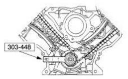
**STEP 8:** Install the crankshaft sprocket with the flange facing forward.
