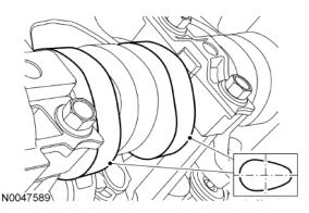
**STEP 9: NOTE:** Do not allow the valve keepers to fall off of the valve or the valve may drop into the cylinder. If a valve drops into a cylinder, the cylinder head must be removed. For additional information, refer to Cylinder Head in this section.
