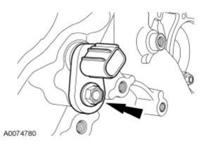
**STEP 11:** Connect the CMP electrical connector.
