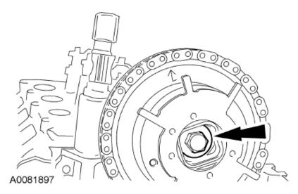
**STEP 16:** Inspect the camshaft phaser and sprocket for damage. For additional information, refer to Camshaft Phaser and Sprocket in this section.
