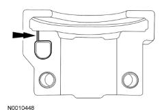
STEP 15: CAUTION: Damage to the camshaft phaser and sprocket assembly will occur if mishandled or used as a lifting or leveraging device.
