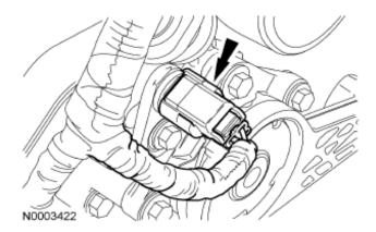
**STEP 5:** Remove the bolt and the RH CMP sensor.
