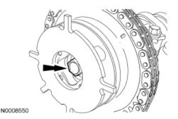
**STEP 16:** Inspect the camshaft phaser and sprocket for damage. For additional information, refer to Camshaft Phaser and Sprocket in this section.
