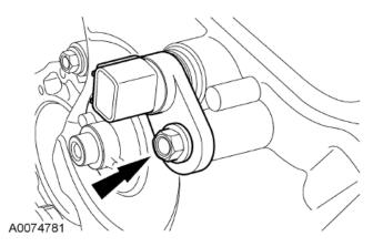
**STEP 11:** Connect the CMP electrical connector.
