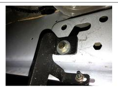
**Step 11:** There will be ½" of adjustment in the (x3) mounting bracket. Adjust to desired position and tighten to (20 ft,/lbs).
