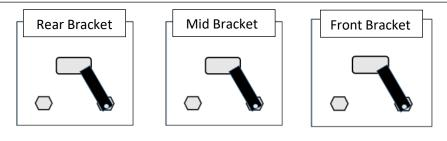
U-clip positioning. NOTE: Clips will also face forward for passenger side.
