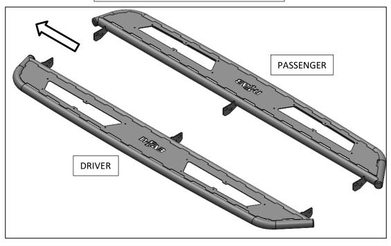
**Step 2:** Install the supplied step plate (x2) to each Running Board using the M6x20mm button head bolts, M6 nuts and M6 flat washer. \*\*\*\* DO NOT OVER TIGHTEN \*\*\*\*
