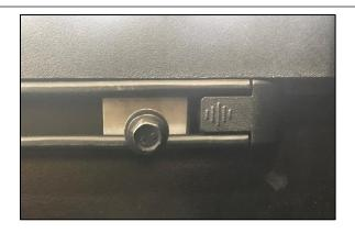
**<u>Step 4.</u>** Next, slide the two remaining bolt and nut assemblies half way through the channel.
