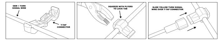
3. Install Horn, Controller and Switch Panel: Mount the horn, controller and switch panels onto proper locations and securely connect them based on the diagram on the last page. Following the below steps and use the included Solderless & Crimp-less Heat Shrink Butt Terminal to connect extension wires if needed.
