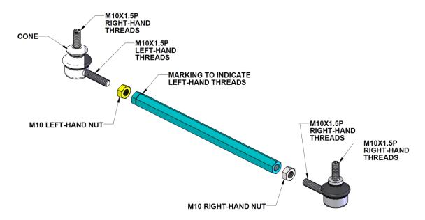
7. Attach Dinan end links to the strut using the 10mm nylon locknuts. Note that the ball joint with the tapered seat attaches to the strut.
