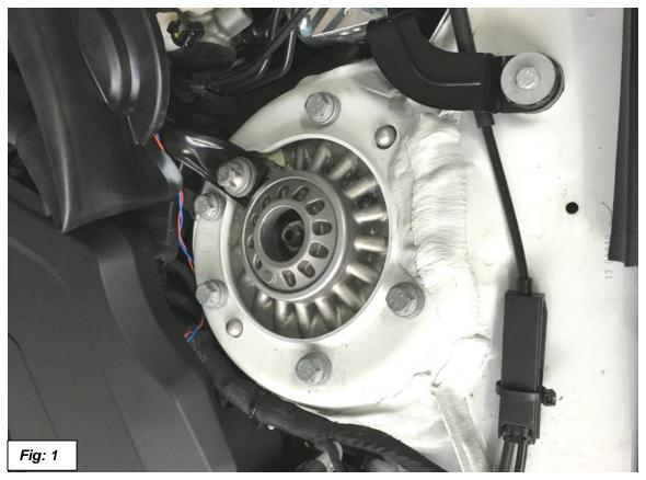
4. Reuse the paper gasket that goes between the body and the camber plate. See Figure 2.
