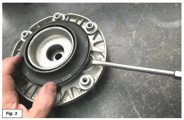
6. Install spring perch bearing on the Dinan slide camber plate. See Figure 4.
