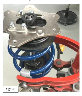
10. Line up the holes, and use the supplied M8x12 socket head cap screws and washers to attach the strut assembly to the body. Torque bolts to 20 ft-lbs. Do not use an impact!
