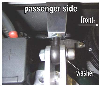
At this point all the pieces should be installed in position with none of the hardware tightened.
