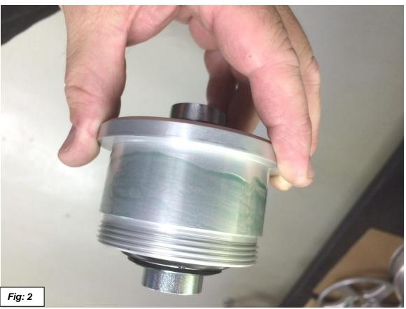
4. See figure below. Slide the carrier into the bore in the arm with a slight turning motion to further spread the Loctite around. Slide the Balljoint Holder Assy into the chamfer side of the arm. See Figure 3.
