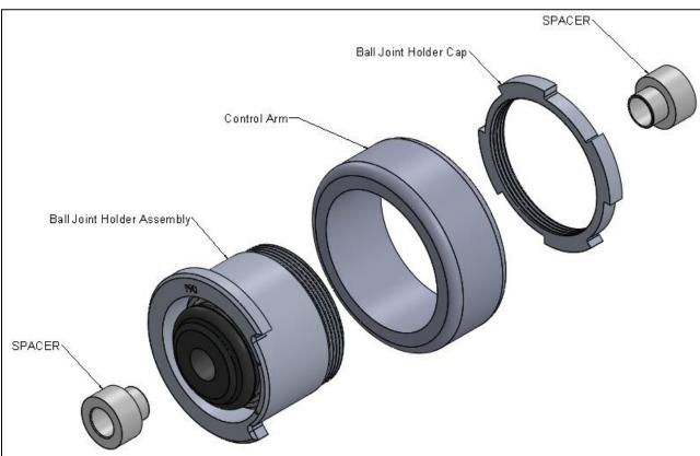
5. Install the Dinan retaining cap onto the arm. Put a small amount of Loctite on the internal threads of the cap and torque to 110 foot-pounds to secure the retaining cap. A special Dinan cap tool is included in every kit. This tool is used with a 1/2" torque drive. Set torque wrench to 110 foot-pounds and do not concern yourself with a conversion factor. See figure below.
