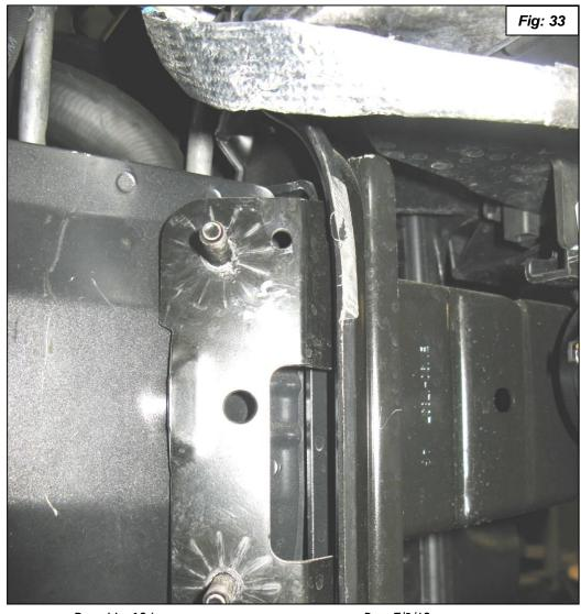
24. Remove the top support bracket from the stock oil cooler. The screws are tamper proof torx. If you do not have the correct tool to remove them, vise grip pliers will work in a pinch. See **figure 34**.
