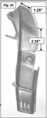
19. Clamp the rivet supports on the brake duct as shown in figures21, 22 and 23 and drill the holes with a 1/8" drill bit.
