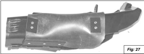
21. Trim the extra  $\frac{1}{2}$ " of rubber close to the rivet supports as shown in **figure 28**.
