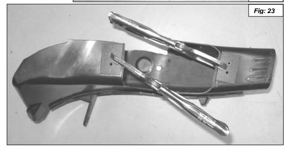
20. Rivet the rubber cover to the brake duct as shown in Figure 24 thru 27. Start as shown in figure 24 and work your way around the duct. Align the edge with the seam. Leave ½" extra rubber at the end.
