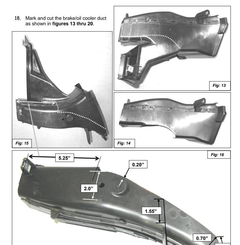
The marked lines show where to cut the oil cooler duct away from the brake duct. A die grinder with a cut off wheel, a hack saw or a razor knife work to cut the duct.
