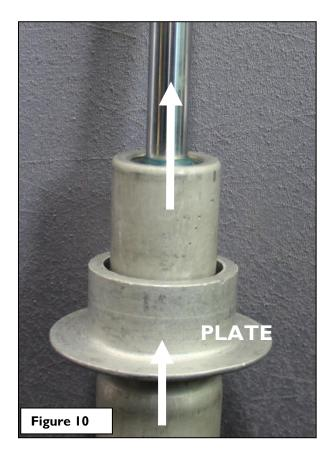
20. Install rear sleeve from Rear Threaded Perch Assy. Use the same procedure as removal of perch plate for install. The part is a press-fit. See Figures 11 & 12.
