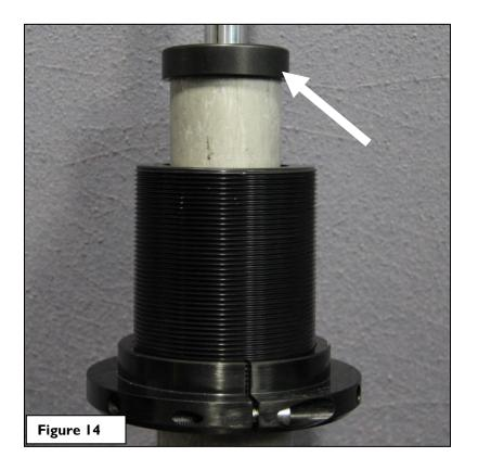
23. Leave the spring perch in the lowest position with the screw loose.
