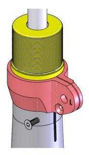
12. Install the spring perch and black plastic isolator disc (in Coil-Over Hardware Kit) as shown. Adjust the perch to about 1/2" up from bottom. This will be the starting ride height setting, and should get you very close to Dinan's target bumpstop clearance measurement. Snug the 6mm screw to lock the perch into place.
